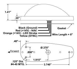
NOTE: Connecting the SYNC (Yellow) wires together will cause those lights to flash at the same time. If synchronization is not necessary or desired, the connection may be left open.
