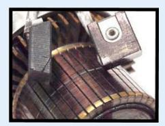
Actual photo of armature commutator and NAASCO's ETR<sup>TM</sup> brushes removed from unit overhauled with our advance ETR-20<sup>TM</sup> improvements. After 1067.3 hours of service, armature commutator wear measured at .003"
