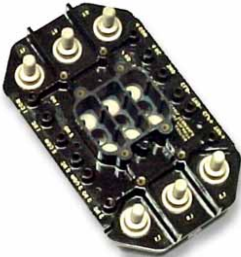
REPAIRED TERMINAL BOARD P/N 977J237
