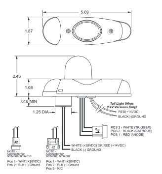
the existing ground lead to the GROUND wire on the input cable assembly or use the supplied connector as shown in the illustrations. Both leads must be connected by an approved FAA connection. Insure that the wire leads clear of any obstructions and ty-wrap as required. Connect the strobe, J1, to the strobe power supply as shown in the figure.
